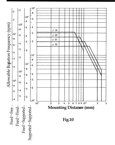
■ Allowable Rotation Frequency (N<sub>c</sub>) and Critical Speed
