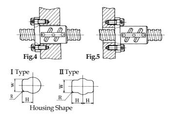
For nut mounting of RBSM Series which method of ball return is by return tube, please design a relief in the housing as shown above to avoid interference with the tube projection.
