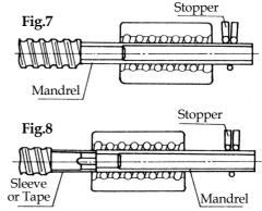
The UZAR RBSW series is shipped with both the nut and screw shaft already assembled. Use the following remover when the nut must be removed from the screw shaft for machining of the end of the shaft. Use the same tool for the nut's assembly. If the remover is not used, the steel balls may fall out of the nut.
